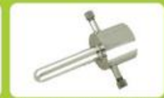
Sealed Atmosphere Chamber
